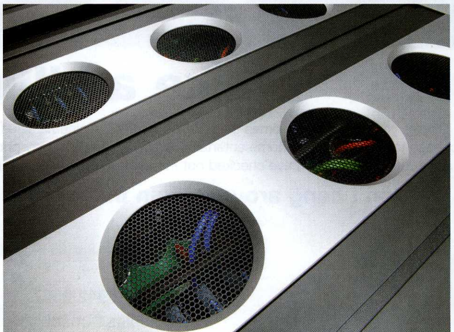
RIGHT: The massive aluminium top plate of the Titan amplifier section is ported to aid cooling. We would have shown you more of the case but it was just too big to fit on the page...
